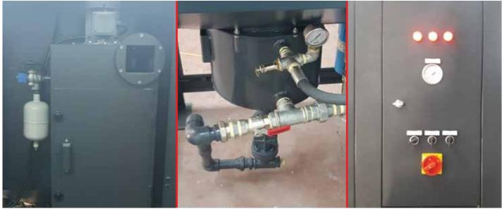
Pressure Sandblasting Machine, Front Loading, Saykar design, has high processing capacity with compact design of small area usage. Motor protected, adjustable pressure and phase display. This pressure sandblasting machine with wide cabin dimensions is suitable for the preparation of surfaces such as wheels and pans.
